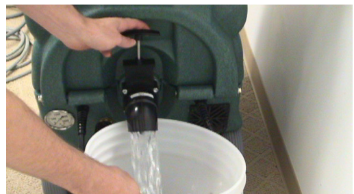
Draining the Recovery Tank
